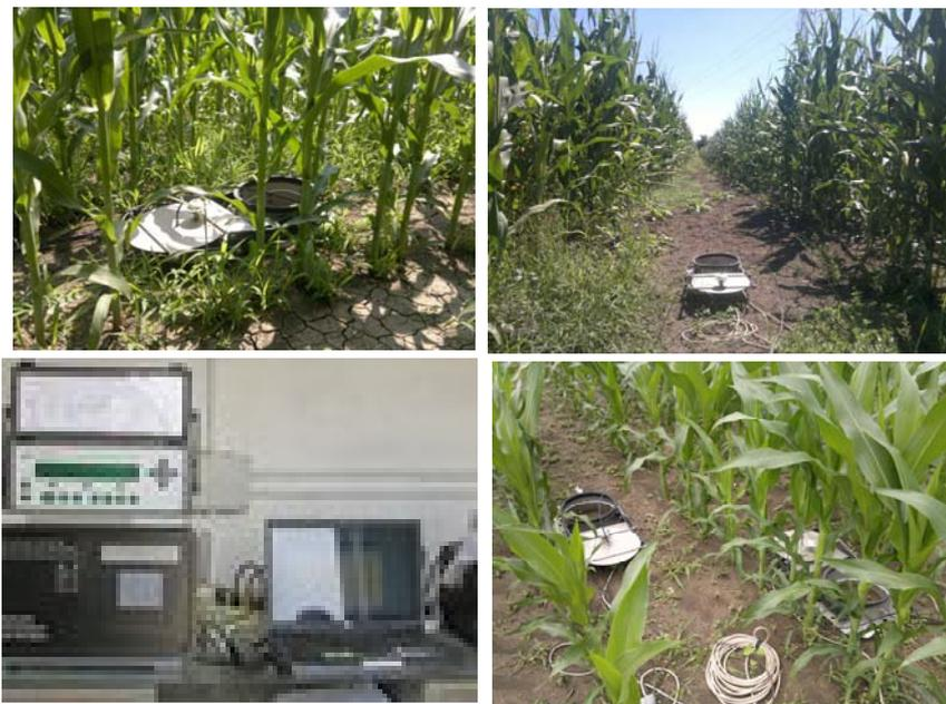
Figure 1 Field chambers and GHG sampling photoacoustic systems
