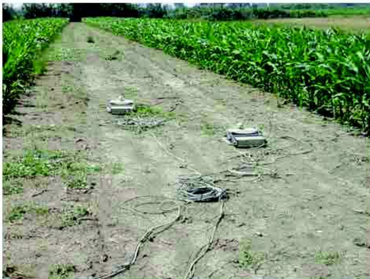
Figure 1. GHG field sampling system
